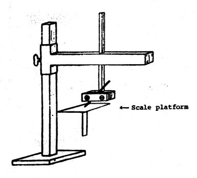
FIGURE 1 - Apparatus for determination of point strength
