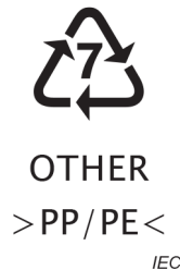
Figure 2 – Marking of polypropylene-polyethylene copolymer battery components
