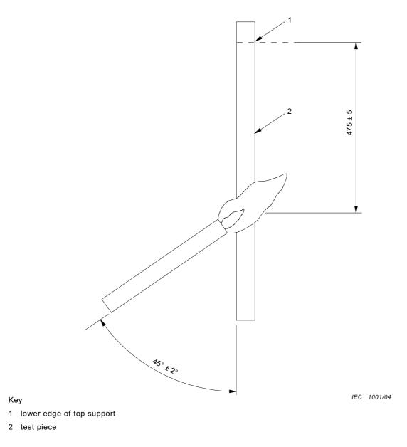
Figure 2 – Application of flame to test piece
