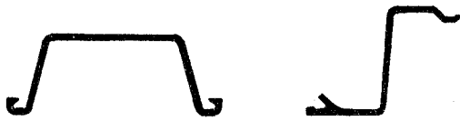
(a) U and Z sheet piling
