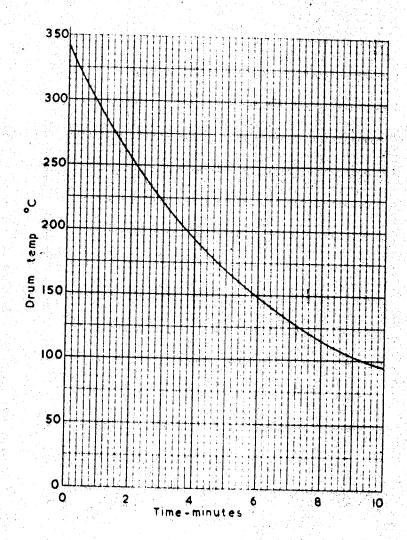
Fig. 4. Standard drum cooling curve, friction materials test machine
