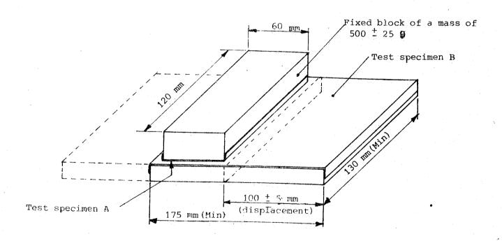
Base plate provided with an arrangement for reciprocating movement
