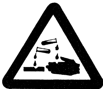
FIGURE - Safety sign to indicate corrosive nature
