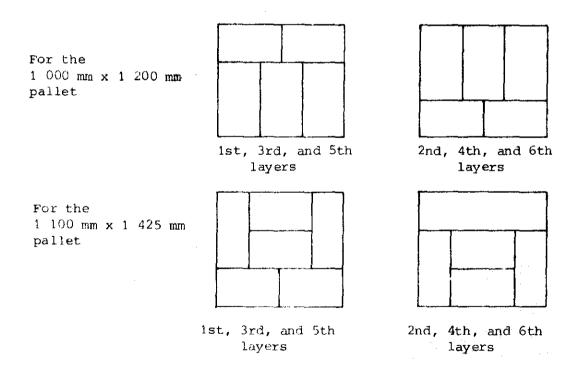
FIGURE 2 - Pattern of stacking bales
