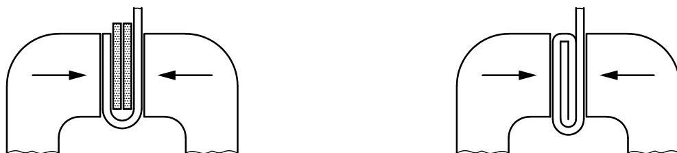
a) Bending with panels as distance pieces (example 2T) b) Bending method with a bench vice (example 2T)
