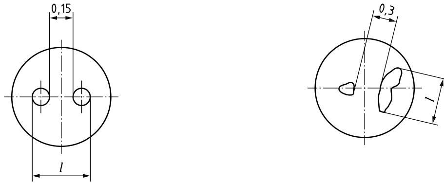
a) Distance between the single defects \leq 0,2 mm
