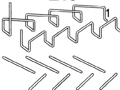
This stitch type is formed with one needle thread (1), which is passed horizontally through the material or through portions of the material and emerges on the same side. All passes of the thread are at an acute angle to the direction of successive needle penetrations, which are in line with the direction of stitching.
