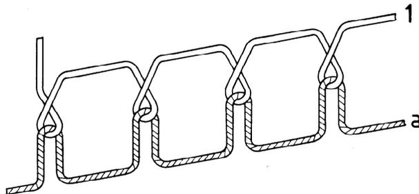
This stitch type is formed with two threads: one needle thread (1) and one bobbin thread (a). A loop of thread 1 is passed through the material from the needle side and is interlaced with thread a on the other side. Thread 1 is pulled back so that the interlacing comes midway between the surfaces of the material being sewn.
