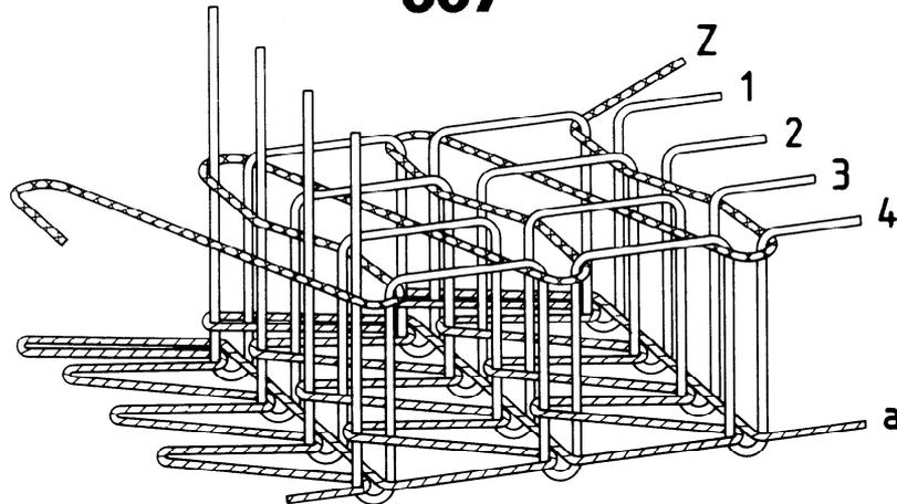
This stitch type is formed with six threads: four needle threads (1, 2, 3 and 4), one looper thread (a) and one cover thread (Z). Loops of threads 1, 2, 3 and 4 are passed through loops of thread Z already laid across the needle side of the material, through the material, and through four separate loops of thread a. They are then interlooped with a further loop of thread a, and the interloopings are drawn against the material.
