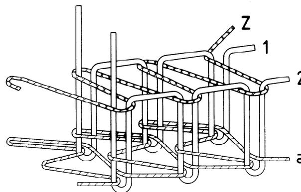
This stitch type is formed with four threads: two needle threads (1 and 2), one looper thread (a) and one cover thread (Z). Loops of threads 1 and 2 are passed through loops of thread Z already laid across the needle side of the material, through the material, and through two separate loops of thread a. They are then interlooped with a further loop of thread a and the interloopings are drawn against the material.
