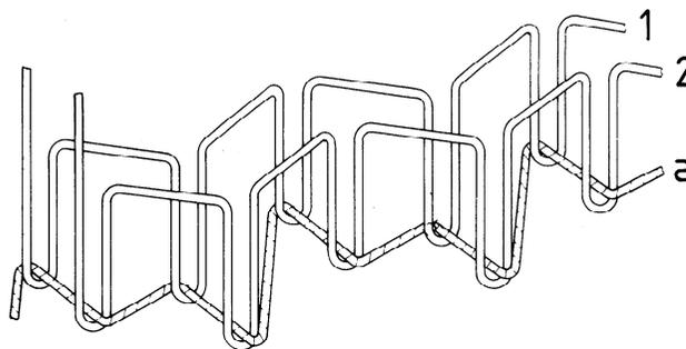
This stitch type is formed with three threads: two needle threads (1 and 2) and one bobbin thread (a). Loops of threads 1 and 2 are passed through the material from the needle side and interlaced with thread a on the other side.
