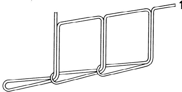
This stitch type is formed with one needle thread (1), a loop of which is passed through the material from the needle side and intralooped in the other side.
