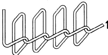
This stitch type is formed with one needle thread (1), which is passed through the material twice, emerging in a position at right-angles to the direction of successive stitch formation, and passing over the thread from the previous stitch forming a loop.
