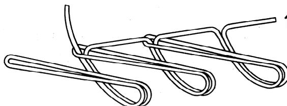
This stitch type is formed with one needle thread (1), a loop of which is passed into the material from the needle side, through portions of the material, emerging on the needle side where it is intralooped at the next point of needle penetration.
