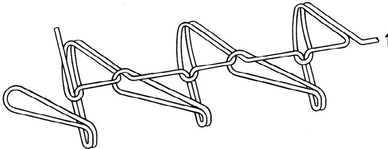
This stitch type is formed with one needle thread (1), a loop of which is passed into the material from the needle side, through portions of the material, emerging on the needle side where it is intralooped at the next point of needle penetration on the axis of stitch formation.
