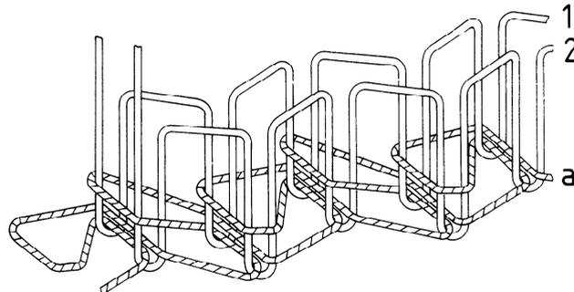
This stitch type is formed with three threads: two needle threads (1 and 2) and one looper thread (a). Loops of threads 1 and 2 are passed through the material from the needle side, and through one loop of thread a on the other side. They are then interlooped with a second loop of thread a. The interloopings are drawn against the material.
