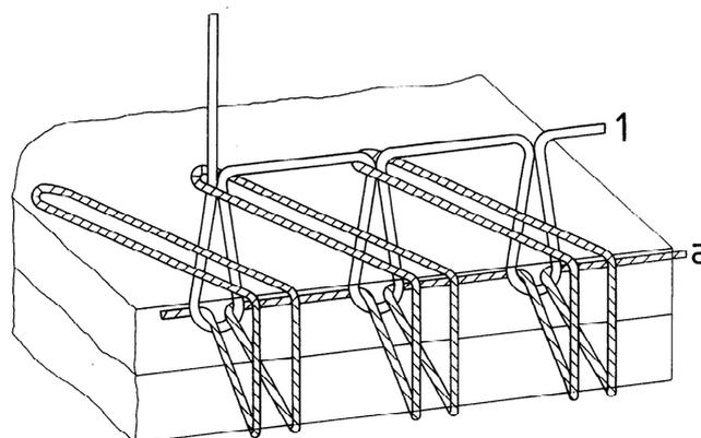
This stitch type is formed with two threads: one needle thread (1) and one looper thread (a). A loop of thread 1 is passed through a loop of thread a already laid across the needle side of the material and through the material. The loop of thread 1 is interlooped with a second loop of thread a at the point of emergence on the other side of the material. The loop of thread a is brought around the edge of the material and extended to the next point of needle penetration.
