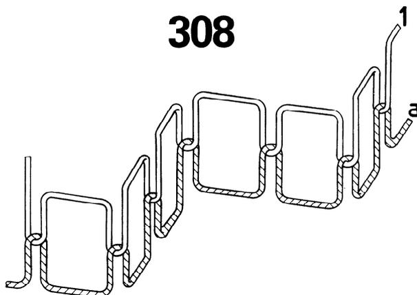
This stitch type is formed with two threads: one needle thread (1) and one bobbin thread (a). A loop of thread 1 is passed through the material from the needle side and is interlaced with thread a on the other side. Thread 1 is pulled back so that the interlacing comes midway between the surfaces of the material.
