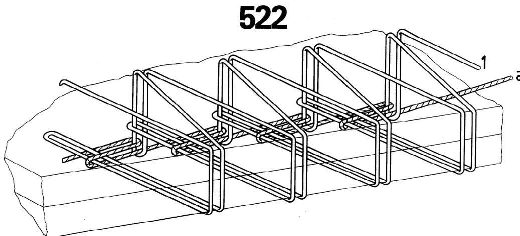
This stitch type is formed with two threads: one needle thread (1) and one looper thread (a). A loop of thread 1 is passed through the material from the needle side and through a second loop of thread 1, and is interlooped with thread a on the other side. This second loop of thread 1 has been brought around the edge of the material to the other side and also interlooped with thread a.
