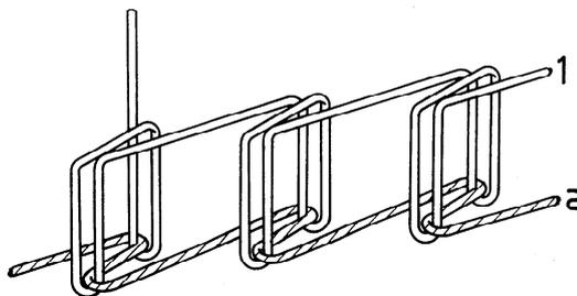
This stitch type is formed with two threads: one needle thread (1) and one bobbin thread (a). A loop of thread 1 is passed through the material from the needle side and is interlaced with thread a on the other side.
