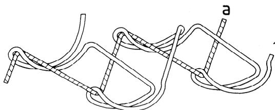
This stitch type is formed with two threads: one needle thread (1) and one bobbin thread (a). A loop of thread 1 is passed into the material from the needle side through portions of the material, emerging on the needle side where it is interlaced with thread a.
