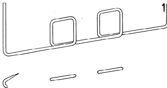
This stitch type is formed with one needle thread (1), which is passed through the material, brought forward a suitable length, passed back through the material and brought back one-third of the initial length before passing again through the material.
