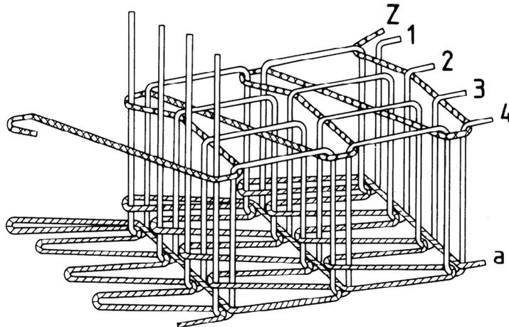
This stitch type is formed with six threads: four needle threads (1, 2, 3 and 4), one looper thread (a) and one cover thread (Z). Loops of threads 1, 2, 3 and 4 are passed through loops of thread Z already laid across the needle side of the material, through the material, and through four separate loops of thread a. They are then interlooped with a further loop of thread a, and the interloopings are drawn against the material.
