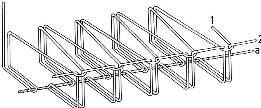
This stitch type is formed with three threads: two needle threads (1 and 2) and one bobbin thread (a). A loop of thread 2 is passed firstly through a loop of thread 1 already laid across the needle side of the material and then through the material. A loop of thread 1 is passed through the material. The loops of threads 1 and 2 are interlaced with thread a at a position midway between the points of emergence on the other side of the material.
