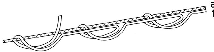
This stitch type is formed with two threads: one needle thread (1) and one bobbin thread (a). A loop of thread 1 is passed into the material from the needle side through portions of the material, emerging on the needle side where it is interlaced with thread a. Needle penetrations are in line with the direction of successive stitch formation.
