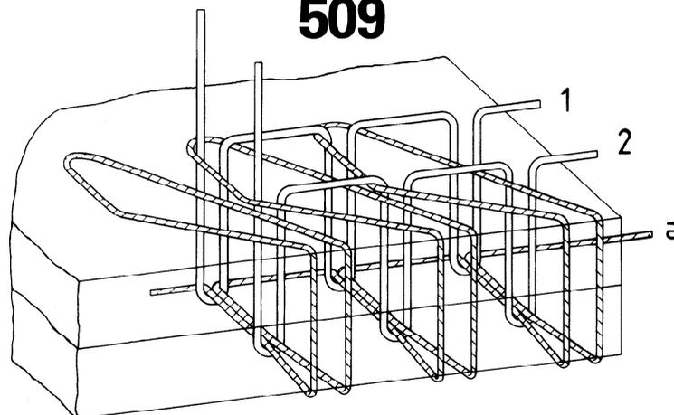
This stitch type is formed with three threads: two needle threads (1 and 2) and one looper thread (a). Loops of threads 1 and 2 are passed through a loop of thread a already laid across the needle side of the material and through the material. The loops of threads 1 and 2 are interlocked with a second loop of thread a at the points of emergence on the other side of the material. The loop of thread a is brought round the edge of the material and extended to the next points of needle penetration.
