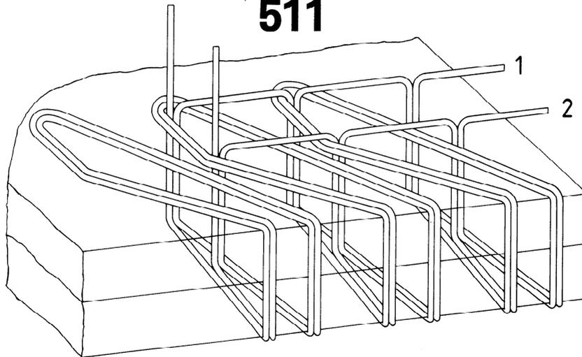
This stitch type is formed with two needle threads (1 and 2). Loops of threads 1 and 2 already laid across the needle side of the material, and through the material. The loops are then brought around the edge of the material and extended to the next points of needle penetration.
