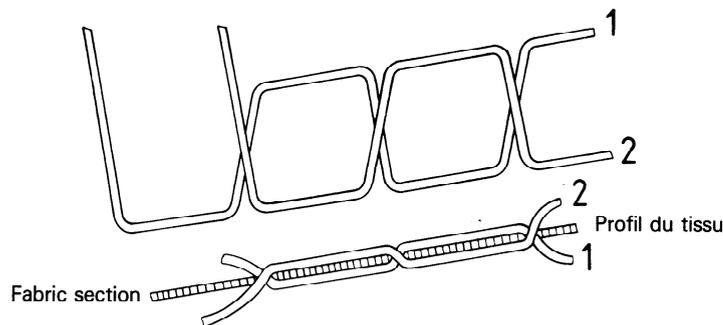
This stitch type is formed with two needle threads (1 and 2), which are passed through the material, through the same perforation from opposite directions, without interlacing or interlooping. They are then brought forward a suitable length and passed back through the material, from opposite directions, through another perforation without interlacing or interlooping.
