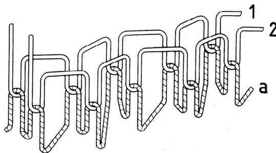
This stitch type is formed with three threads: two needle threads (1 and 2) and one bobbin thread (a). Loops of threads 1 and 2 are passed through the material from the needle side and interlaced with thread a on the other side. Threads 1 and 2 are pulled back so that the interlacings come midway between the surfaces of the material.
