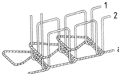
This stitch type is formed with three threads: two needle threads (1 and 2) and one looper thread (a). Loops of threads 1 and 2 are passed through the material from the needle side, and through one loop of thread a on the other side. They are then interlooped with a second loop of thread a. The interloopings are drawn against the material.
