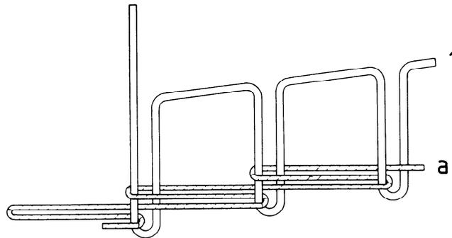
This stitch type is formed with two threads: one needle thread (1) and one looper thread (a). A loop of thread 1 is passed through the material from the needle side, and through one loop of thread a on the other side. It is then interlooped with a second loop of thread a. The interloopings are drawn against the material.
