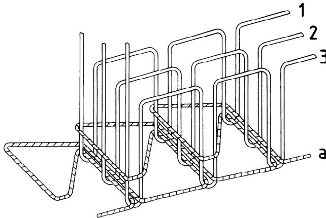
This stitch type is formed with four threads: three needle threads (1, 2 and 3) and one looper thread (a). Loops of threads 1, 2 and 3 are passed through the material from the needle side, and through one loop of thread a on the other side. They are then interlooped with a second loop of thread a. The interloopings are drawn against the material.
