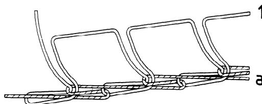
This stitch type is formed with two threads: one needle thread (1) and one looper thread (a). A loop of thread 1 is passed into the material from the needle side, through portions of the material, emerging on the needle side. It is passed through one loop of thread a, and is then interlooped with a second loop of thread a. Needle penetrations are at right-angles to the direction of successive stitch formation.
