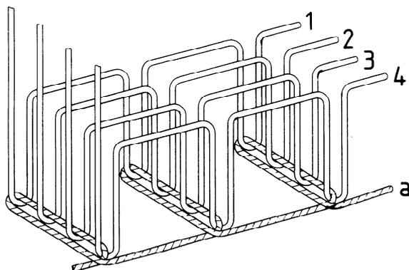
This stitch type is formed with five threads: four needle threads (1, 2, 3 and 4) and one bobbin thread (a). Loops of threads 1, 2, 3 and 4 are passed through the material from the needle side and interlaced with thread a on the other side.
