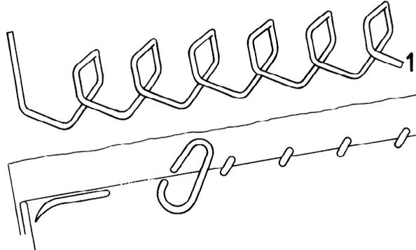
This stitch type is formed with one needle thread (1), which is passed through the fold of material and into the single material a short distance above and slightly to the right. The thread is then passed diagonally back through both material layers to a point in line with the previous point of thread emergence.
