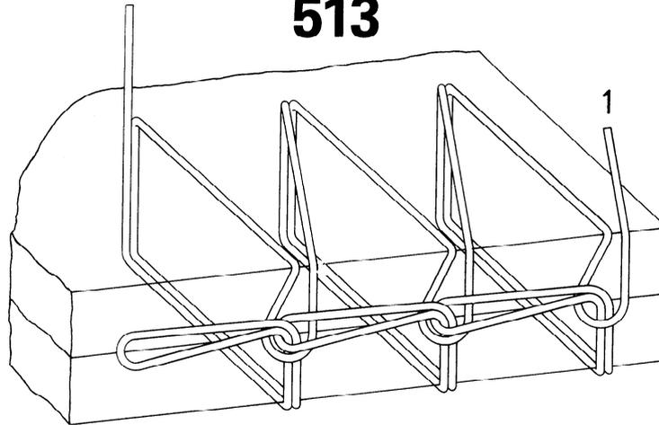
This stitch type is formed with one needle thread (1). A loop of this thread is passed through the material from the needle side and brought to the edge of the material where it is interlooped with a second loop which has been drawn across the needle side to the edge of the material, and with a further loop from the previous stitch.
