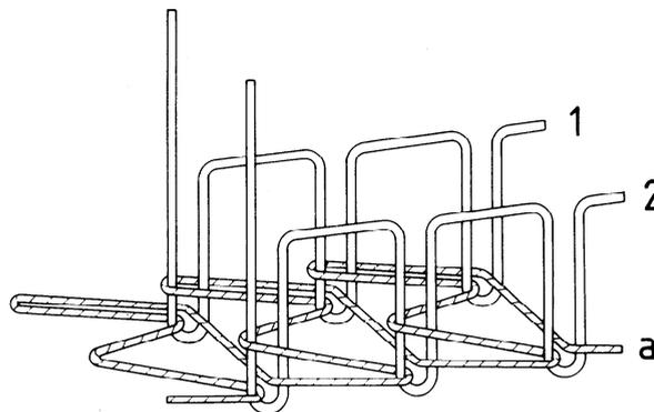
This stitch type is formed with three threads: two needle threads (1 and 2) and one looper thread (a). Loops of threads 1 and 2 are passed through the material from the needle side, and through two separate loops of thread a on the other side. They are then interlooped with a further loop of thread a. The interloopings are drawn against the material.
