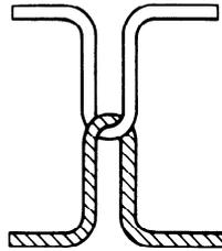
**2.2 stitch type:** An assembly of recurring stitches, relating to the material and which may be characterized by a change in direction. The minimum number of stitches that describe a stitch type is indicated.
