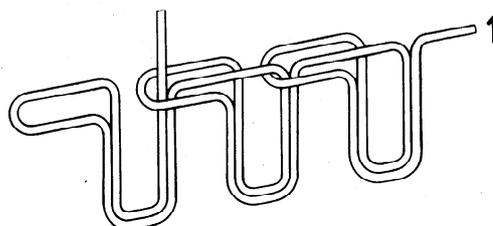
This stitch type is formed with one needle thread (1), a loop of which is passed through the material from the needle side, passed back through the material to the needle side at a distance, and intralooped on the needle side of the material at the next point of needle penetration.
