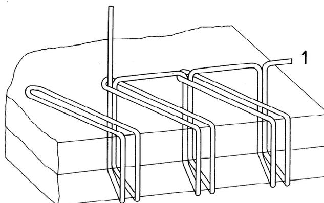
This stitch type is formed with one needle thread (1), a loop of which is passed through a loop of thread 1 already laid across the needle side of the material and through the material. It is brought around the edge of the material and extended to the next point of needle penetration.
