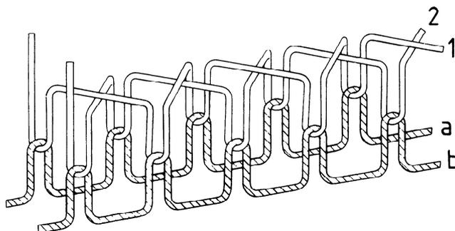
This stitch type is formed with four threads: two needle threads (1 and 2) and two bobbin threads (a and b). Loops of threads 1 and 2 are passed through the material from the needle side and one loop of thread 1 is interlaced with thread a and one loop of thread 2 with thread b on the other side. Threads 1 and 2 are pulled back so that the interlacing comes midway between the surfaces of material.
