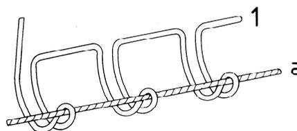
This stitch type is formed with two threads: one needle thread (1) and one bobbin thread (a). A loop of thread 1 is passed into the material from the needle side, through portions of the material, emerging on the needle side where it is interlaced with thread a.
