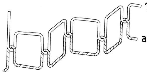
This stitch type is formed with two threads: one needle thread (1) and one bobbin thread (a). A loop of thread 1 is passed through the material from the needle side and is interlaced with thread a on the other side. Thread 1 is pulled back so that the interlacing comes midway between the surfaces of the material being sewn.
