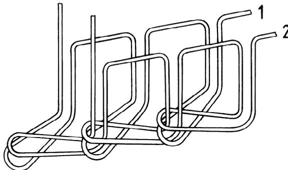
This stitch type is formed with two needle threads (1 and 2), loops of which are passed through the material from the needle side. Thread 2 is intralooped with thread 1 on the other side of the material.
