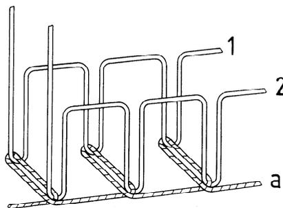
This stitch type is formed with three threads: two needle threads (1 and 2) and one bobbin thread (a). Loops of threads 1 and 2 are passed through the material from the needle side and interlaced with thread a on the other side.
