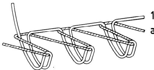
This stitch type is formed with two threads: one needle thread (1) and one bobbin thread (a). A loop of thread 1 is passed through a loop of thread a on the needle side and then into the material, through portions of the material, emerging on the needle side where it is interlaced with thread a. Needle penetrations are at right-angles to the direction of successive stitch formation.
