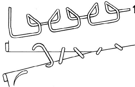
This stitch type is formed with one needle thread (1), which is passed through the folded edge of a material and brought forward a suitable length in the fold before emerging from the material. It is then passed through an opposite folded edge of material at a point slightly behind the point of thread emergence.
