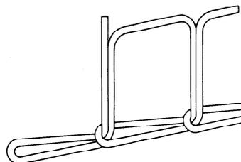
**2.1.2 interlooping:** The passing of a loop of thread through another loop formed by a different thread.
