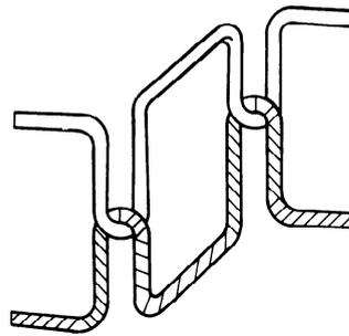
**2.3 group of threads:** A number of threads fulfilling an identical function, for example needle or looper.
