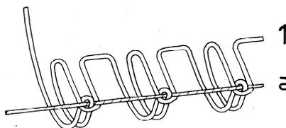
This stitch type is formed with two threads: one needle thread (1) and one bobbin thread (a). A loop of thread 1 is passed into the material from the needle side through portions of the material emerging on the needle side, where it is intralooped, and then interlaced with thread a.
