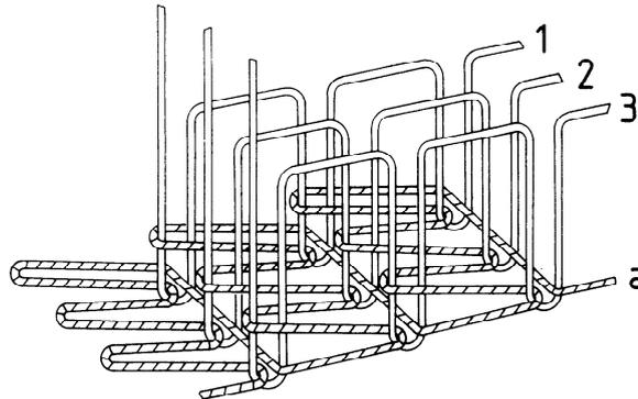
This stitch type is formed with four threads: three needle threads (1, 2 and 3) and one looper thread (a). Loops of threads 1, 2 and 3 are passed through the material from the needle side, and through three separate loops of thread a on the other side. They are then interlooped with a further loop of thread a. The interloopings are drawn against the material.
