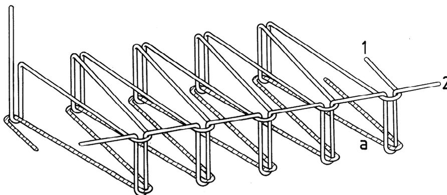
This stitch type is formed with three threads: two needle threads (1 and 2) and one bobbin thread (a). A loop of thread 2 is passed through a loop of thread 1 already laid across the needle side of the material and through the material. A loop of thread 1 is passed through the material. The loops of threads 1 and 2 are interlaced with thread a on the other side.
