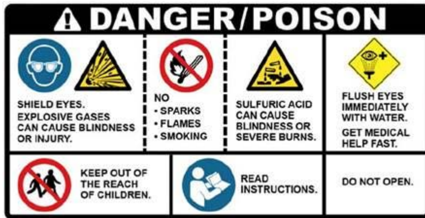
Figure C.3 – Safety labelling – Label for North America area, new version
