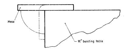
FIGURE 3 - Bending of the Sample
