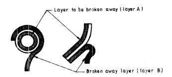
FIGURE 2 - Ring-shaped and strip-shaped test pieces
