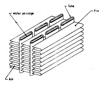
FIGURE 3 - Tube and corrugated fin core
