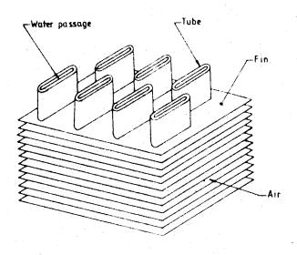
FIGURE 1 - Tube and plate fin core
