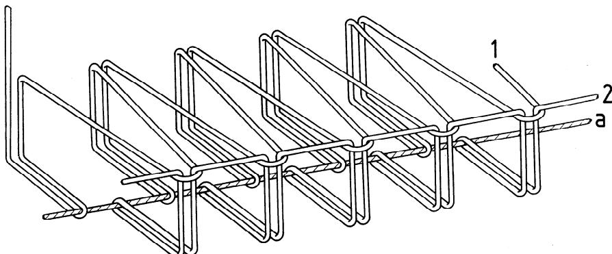
This stitch type is formed with three threads: two needle threads (1 and 2) and one bobbin thread (a). A loop of thread 2 is passed firstly through a loop of thread 1 already laid across the needle side of the material and then through the material. A loop of thread 1 is passed though the material. The loops of threads 1 and 2 are interlaced with thread a at a position midway between the points of emergence on the other side of the material.
