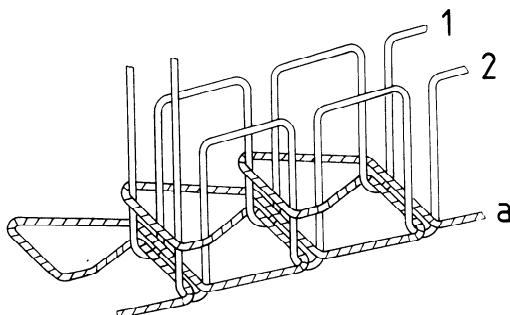
This stitch type is formed with three threads: two needle threads (1 and 2) and one looper thread (a). Loops of threads 1 and 2 are passed through the material from the needle side, and through one loop of thread a on the other side. They are then interlooped with a second loop of thread a. The interloopings are drawn against the material.
