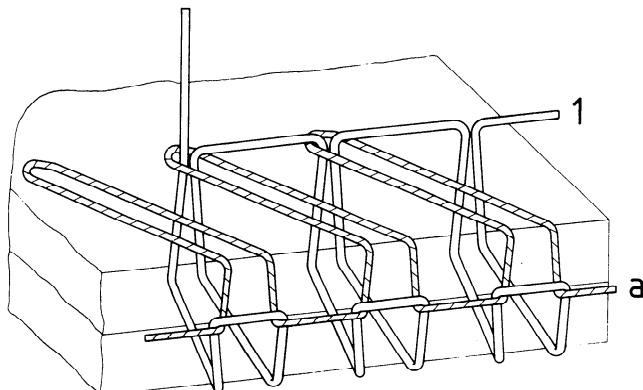
This stitch type is formed with two threads: one needle thread (1) and one looper thread (a). A loop of thread 1 is passed through a loop of thread a already laid across the needle side of the material and through the material. The loop of thread 1 is brought to the edge of the material where it is interlooped with a second loop of thread a. The loop of thread a is extended from this interlooping to the next point of needle penetration.
