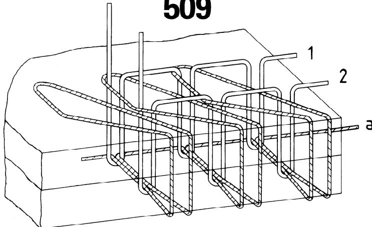
This stitch type is formed with three threads: two needle threads (1 and 2) and one looper thread (a). Loops of threads 1 and 2 are passed through a loop of thread a already laid across the needle side of the material and through the material. The loops of threads 1 and 2 are inter-looped with a second loop of thread a at the points of emergence on the other side of the material. The loop of thread a is brought round the edge of the material and extended to the next points of needle penetration.
