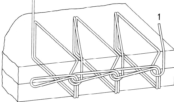
This stitch type is formed with one needle thread (1). A loop of this thread is passed through the material from the needle side and brought to the edge of the material where it is interlooped with a second loop which has been drawn across the needle side to the edge of the material, and with a further loop from the previous stitch.
