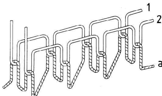
This stitch type is formed with three threads: two needle threads (1 and 2) and one bobbin thread (a). Loops of threads 1 and 2 are passed through the material from the needle side and interlaced with thread a on the other side. Threads 1 and 2 are pulled back so that the interlacings come midway between the surfaces of the material.
