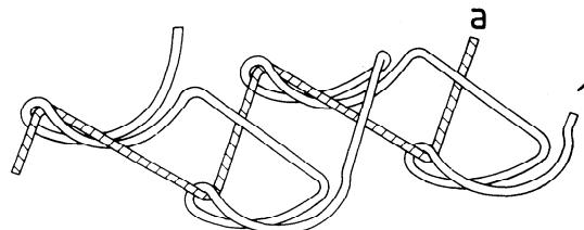
This stitch type is formed with two threads: one needle thread (1) and one bobbin thread (a). A loop of thread 1 is passed into the material from the needle side through portions of the material, emerging on the needle side where it is interlaced with thread a.
