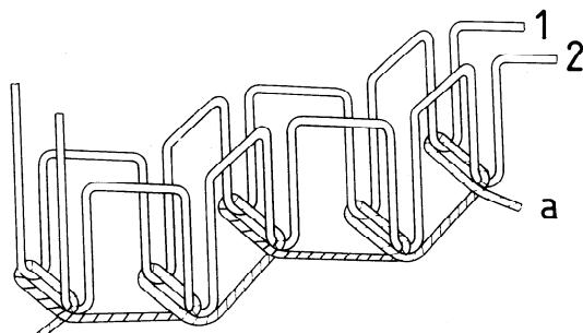
This stitch type is formed with three threads: two needle threads (1 and 2) and one bobbin thread (a). Loops of threads 1 and 2 are passed through the material from the needle side and interlaced with thread a on the other side.
