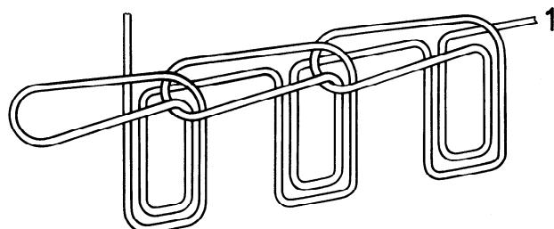
This stitch type is formed with one needle thread (1), a loop of which is passed through the material from the needle side to the other side and passed back through the material to the needle side at a distance. The thread is intralooped where the next loop is passed through the material.
