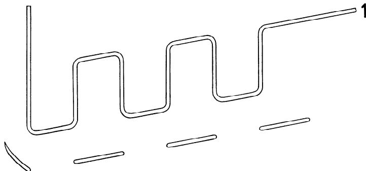
This stitch type is formed with one needle thread (1), which is passed through the material, brought forward a suitable length and passed back through the material.
