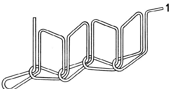
This stitch type is formed with one needle thread (1), a loop of which is passed through the material from the needle side and intralooped on the other side. This stitch type is the same as 101 except that successive single stitches form a symmetrical zigzag pattern.
