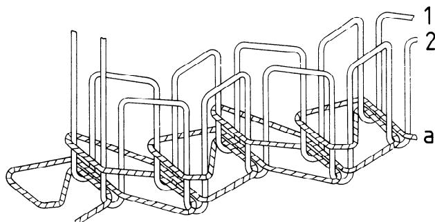
This stitch type is formed with three threads: two needle threads (1 and 2) and one looper thread (a). Loops of threads 1 and 2 are passed through the material from the needle side, and through one loop of thread a on the other side. They are then interlooped with a second loop of thread a. The interloopings are drawn against the material.
