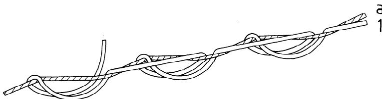
This stitch type is formed with two threads: one needle thread (1) and one bobbin thread (a). A loop of thread 1 is passed through a loop of thread a on the needle side, and then into the material, through portions of the material, emerging on the needle side where it is interlaced with thread a. Needle penetrations are in line with the direction of successive stitch formation.
