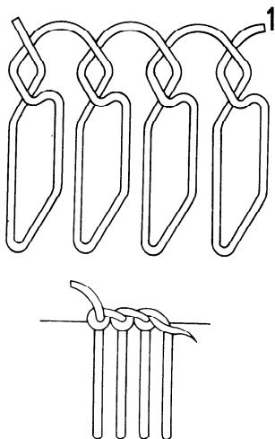
This stitch type is formed with one needle thread (1), which is passed from the material near the cut edge and forward under the material at right-angles to the line of the button-hole, emerging through the material and through a loop of the thread from the previous stitch. The thread is then pulled tight drawing the loop towards the cut edge where the knot is formed.
