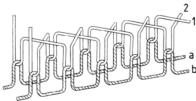
This stitch type is formed with four threads: two needle threads (1 and 2) and two bobbin threads (a and b). Loops of threads 1 and 2 are passed through the material from the needle side and one loop of thread 1 is interlaced with thread a and one loop of thread 2 with thread b on the other side. Threads 1 and 2 are pulled back so that the interlacing comes midway between the surfaces of material.
