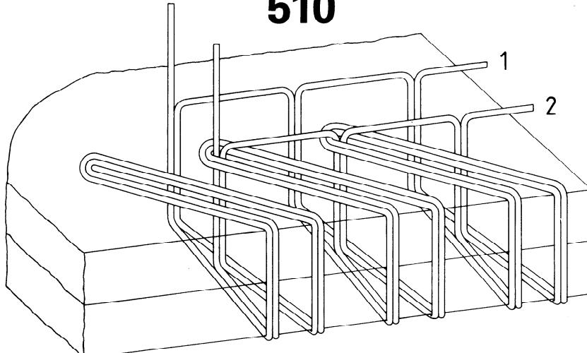
This stitch type is formed with two needle threads (1 and 2). A loop of thread 2 is passed through loops of threads 1 and 2 already laid across the needle side of the material, and through the material. A loop of thread 1 is passed through the material, and the loops of threads 1 and 2 are then brought around the edge of the material and extended to the next point of needle penetration of thread 2.
