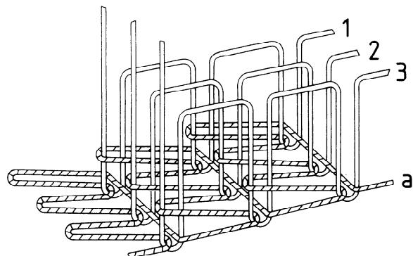
This stitch type is formed with four threads: three needle threads (1, 2 and 3) and one looper thread (a). Loops of threads 1, 2 and 3 are passed through the material from the needle side, and through three separate loops of thread a on the other side. They are then interlooped with a further loop of thread a. The interloopings are drawn against the material.
