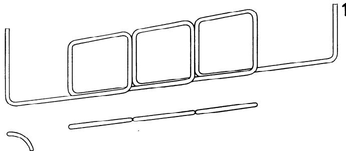
This stitch type is formed with one needle thread (1), which is passed through the material, brought forward a suitable length, passed back through the material and brought back half the initial length before passing back through the material at the point of emergence of the previous thread. This stitch type is often used at the beginning or end of other stitch formations.
