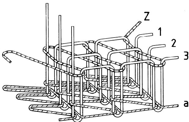
This stitch type is formed with five threads: three needle threads (1, 2 and 3), one looper thread (a) and one cover thread (Z). Loops of threads 1, 2 and 3 are passed through loops of thread Z already laid across the needle side of the material, and then through the material, and through three separate loops of thread a. They are then interlooped with a further loop of thread a and the interloopings are drawn against the material.
