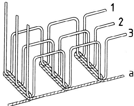
This stitch type is formed with four threads: three needle threads (1, 2 and 3) and one bobbin thread (a). Loops of threads 1, 2 and 3 are passed through the material from the needle side and interlaced with thread a on the other side.
