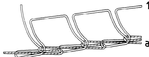
This stitch type is formed with two threads: one needle thread (1) and one looper thread (a). A loop of thread 1 is passed into the material from the needle side, through portions of the material, emerging on the needle side. It is passed through one loop of thread a, and is then interlooped with a second loop of thread a. Needle penetrations are at right-angles to the direction of successive stitch formation.
