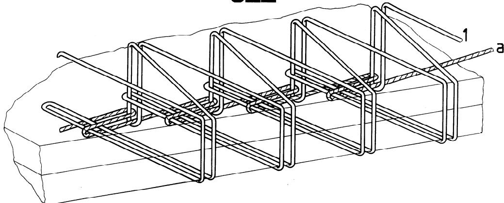
This stitch type is formed with two threads: one needle thread (1) and one looper thread (a). A loop of thread 1 is passed through the material from the needle side and through a second loop of thread 1, and is interlooped with thread a on the other side. This second loop of thread 1 has been brought around the edge of the material to the other side and also interlooped with thread a.
