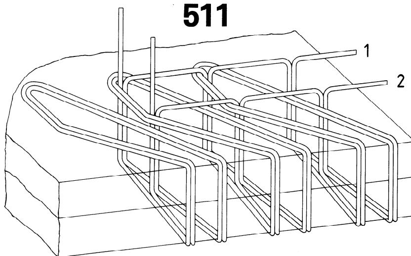
This stitch type is formed with two needle threads (1 and 2). Loops of threads 1 and 2 are passed through loops of threads 1 and 2 already laid across the needle side of the material, and through the material. The loops are then brought around the edge of the material and extended to the next points of needle penetration.
