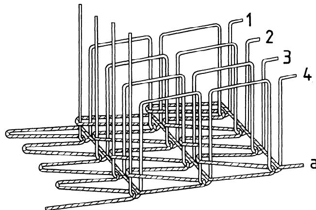
This stitch type is formed with five threads: four needle threads (1, 2, 3 and 4) and one looper thread (a). Loops of threads 1, 2, 3 and 4 are passed through the material from the needle side, and through four separate loops of thread a on the other side. They are then interlooped with a further loop of thread a. The interloopings are drawn against the material.
