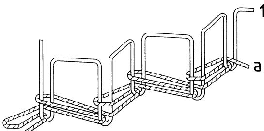
This stitch type is formed with two threads: one needle thread (1) and one looper thread (a). A loop of thread 1 is passed through the material from the needle side, and through one loop of thread a on the other side. It is then interlooped with a second loop of thread a. The interloopings are drawn against the material.
