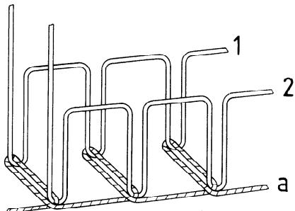
This stitch type is formed with three threads: two needle threads (1 and 2) and one bobbin thread (a). Loops of threads 1 and 2 are passed through the material from the needle side and interlaced with thread a on the other side.
