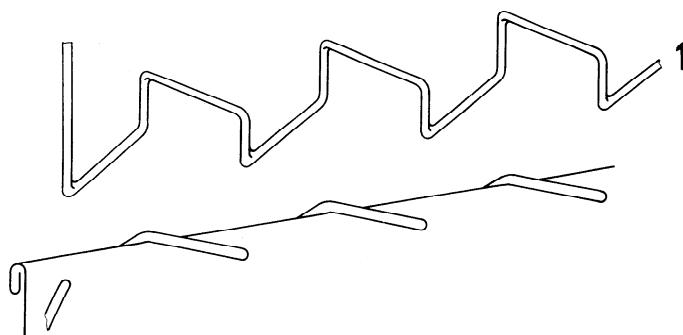
This stitch type is formed with one needle thread (1), which is passed through the material, cast over the rolled edge of the material and brought forward through the material, in line with the previous thread emergence.
