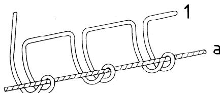
This stitch type is formed with two threads: one needle thread (1) and one bobbin thread (a). A loop of thread 1 is passed into the material from the needle side, through portions of the material, emerging on the needle side where it is interlaced with thread a.
