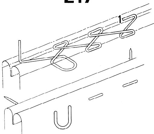
This stitch type is formed with one needle thread (1), which is passed diagonally through the material layers, brought back a suitable length behind the point of emergence, and passed diagonally back through the material, crossing the first diagonal.
