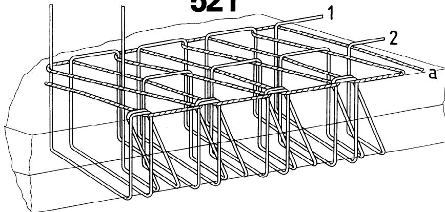
This stitch type is formed with three threads: two needle threads (1 and 2) and one looper thread (a). Loops of threads 1 and 2 are passed through a loop of thread a already laid across the needle side of the material, and through the material. The loops of threads 1 and 2 are brought to the edge of the material where they are interlooped with a second loop of thread a. The loop of thread a is extended from this interlooping to the next points of needle penetration.
