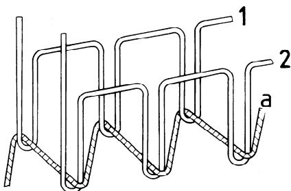
This stitch type is formed with three threads: two needle threads (1 and 2) and one bobbin thread (a). Loops of threads 1 and 2 are passed through the material from the needle side and interlaced with thread a on the other side.
