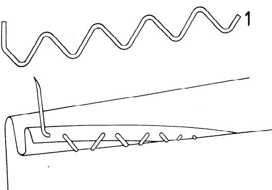
This stitch type is formed with one needle thread (1), which is passed through the single material, passed forward through the turned over edge of the hem (turned back for the purpose), emerging slightly in front, in line with the previous thread penetration and taking up a very small amount of the material; the thread is then brought forward and through the material below the hem to repeat the stitch. Very small amounts of material are taken up.
